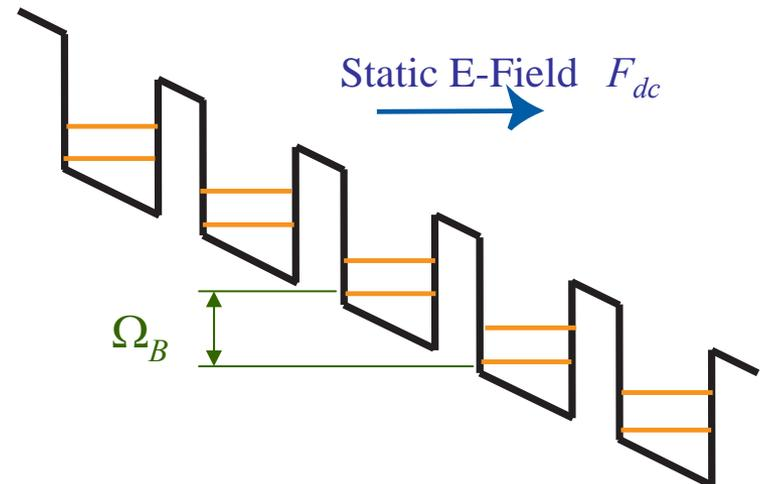
$$\text{Bloch Frequency: } \Omega_B = eF_{dc}d$$
