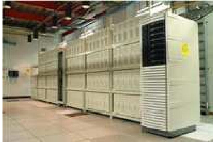
128 node dual 2.4GHz P4 Myrinet cluster, commissioned at FNAL in January 2003
