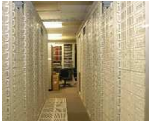
128 node dual 2.4GHz P4 Myrinet cluster, commissioned at FNAL in January 2003
