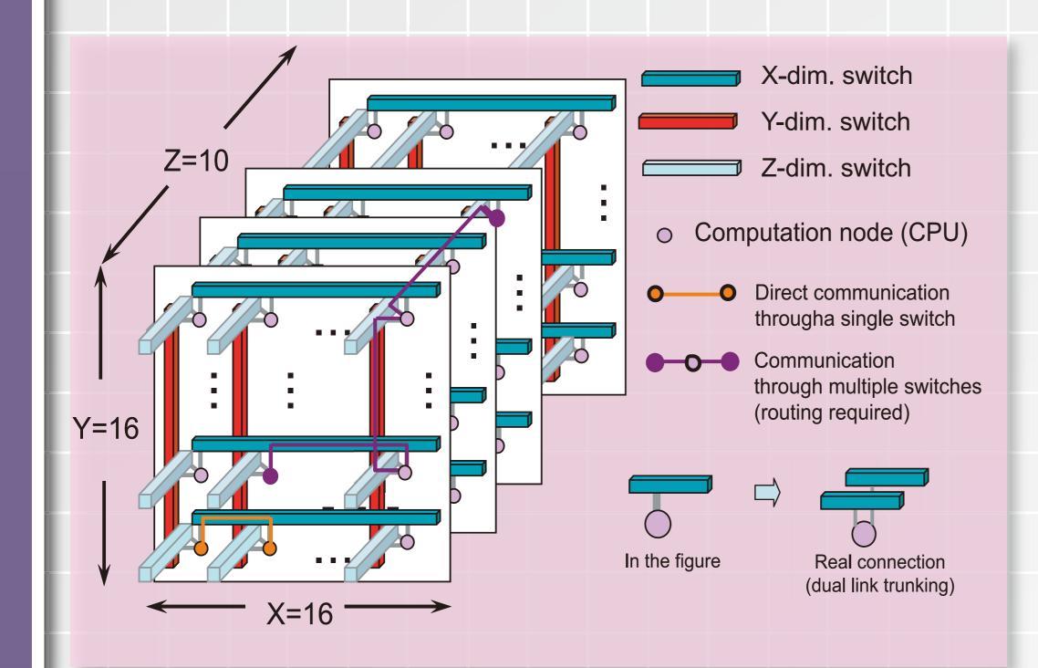
A computation node is equipped with three (X-, Y- and Z-dimension) of paired on-board GbE NICs (6 ports in total) for data communication. Nodes on a single line of a dimension are connected by an L2 GbE switch. For 3-D nearest neighboring communication, the node can communicate with surrounding nodes simultaneously with aggregated 750MB/s of theoretical peak bandwidth.
