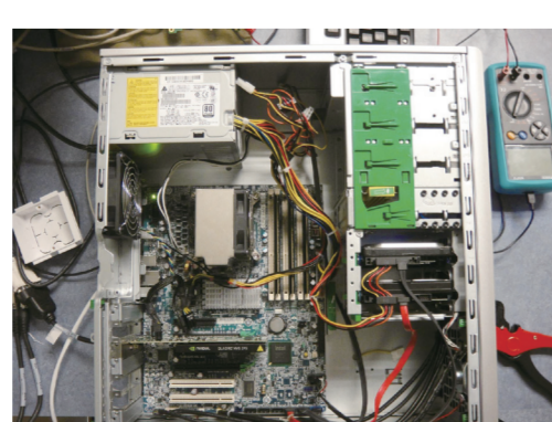
Base system (HP Z400 6-DIMM Edition) Intel Xeon W3505 2.53GHz, DDR-SDRAM 3GB
