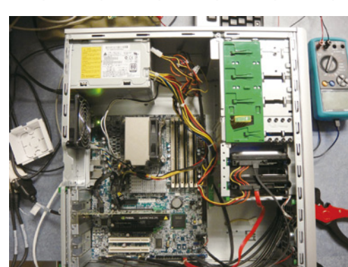
Base system (HP Z400 6-DIMM Edition) Intel Xeon W3505 2.53GHz, DDR-SDRAM 3GB (*) Cooling fans and some components were disconnected for power measurement.
