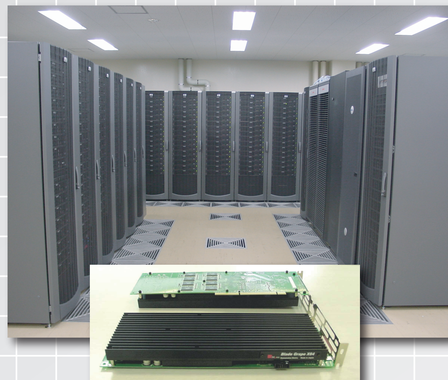
FIRST simulator (256 nodes, 36.1TFLOPS) and Blade-GRAPE board.
