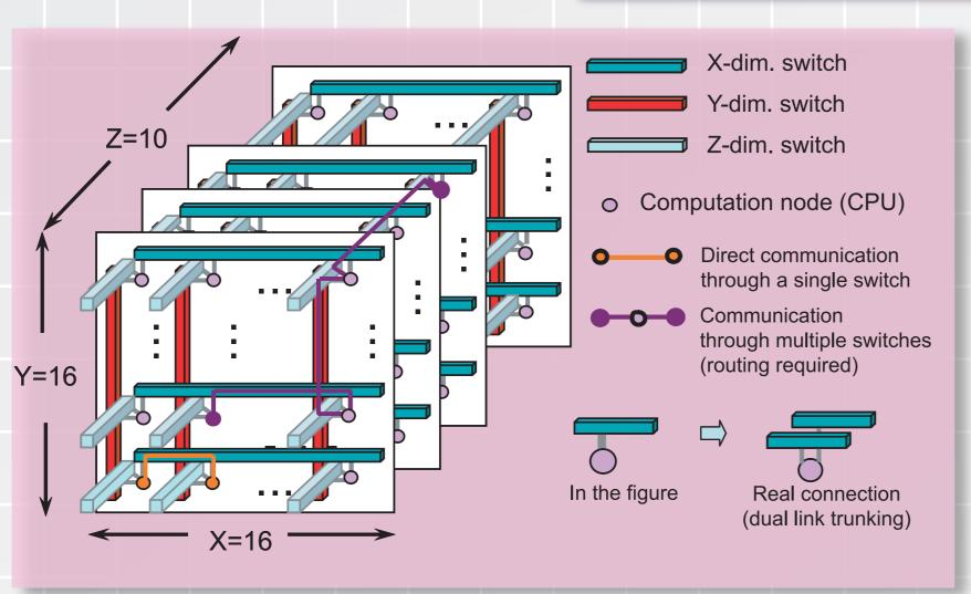
Each computation node is equipped with three (X-, Y- and Zdimension) paired on-board GbE NICs (6 ports in total) for data communication. Nodes on a single line of a dimension are connected by an L2 GbE switch. For 3-D nearest neighboring communication, the node can communicate with surrounding nodes simultaneously with aggregated 750 MB/s of theoretical peak bandwidth.
