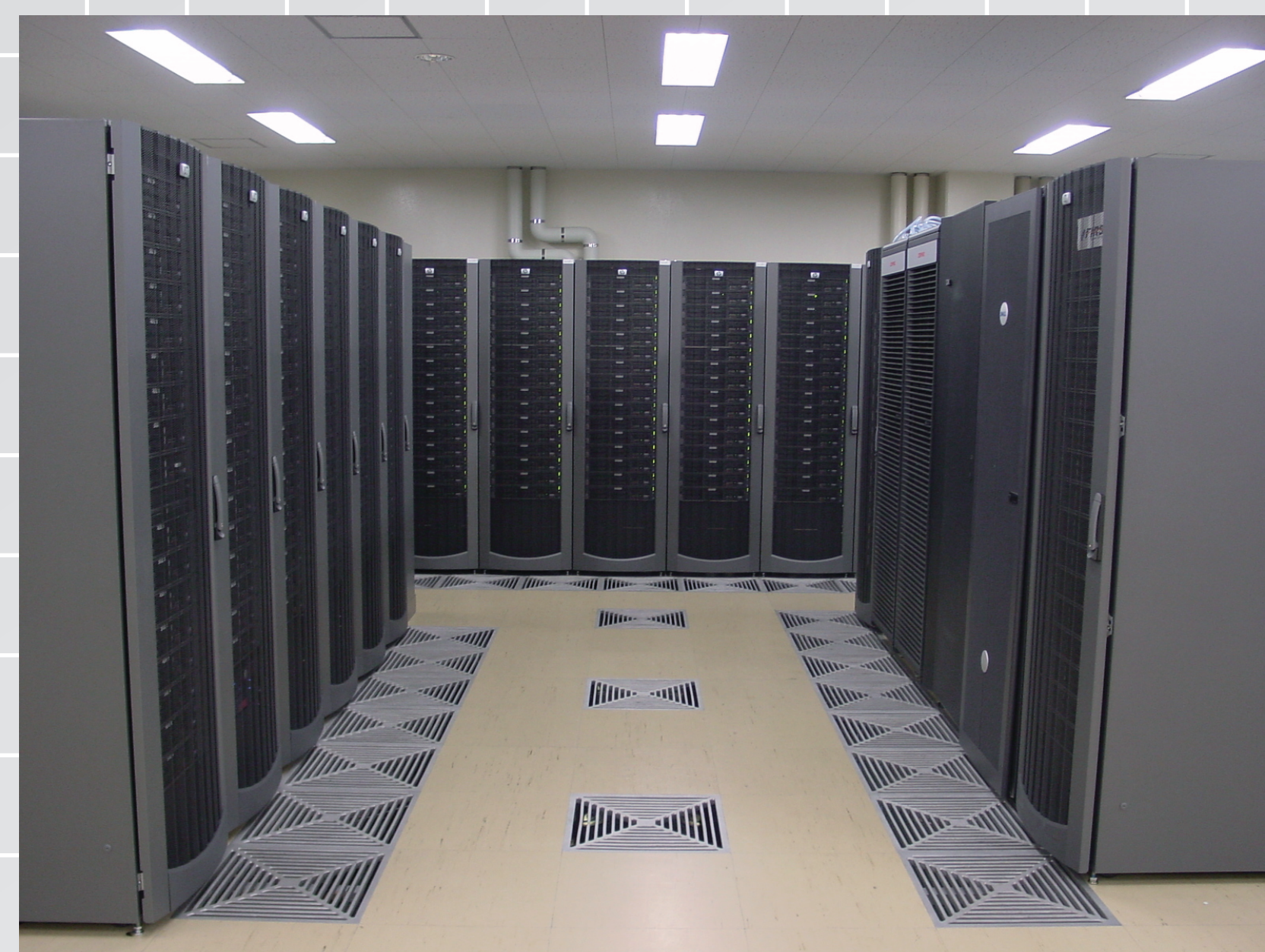
Fig. 1 - The 240 node model of FIRST cluster (33.3TFLOPS).
