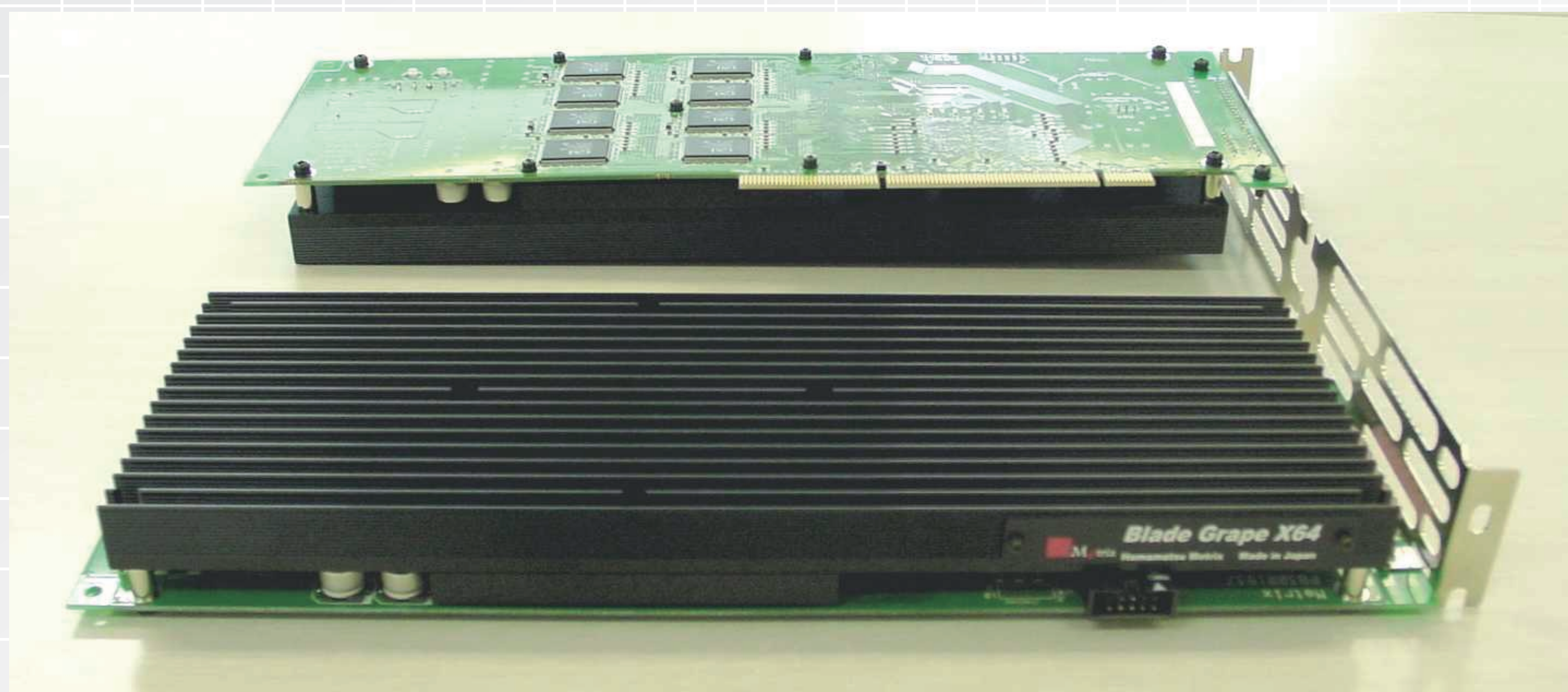
Fig. 2 - Blade-GRAPE board (136.8GFLOPS)
