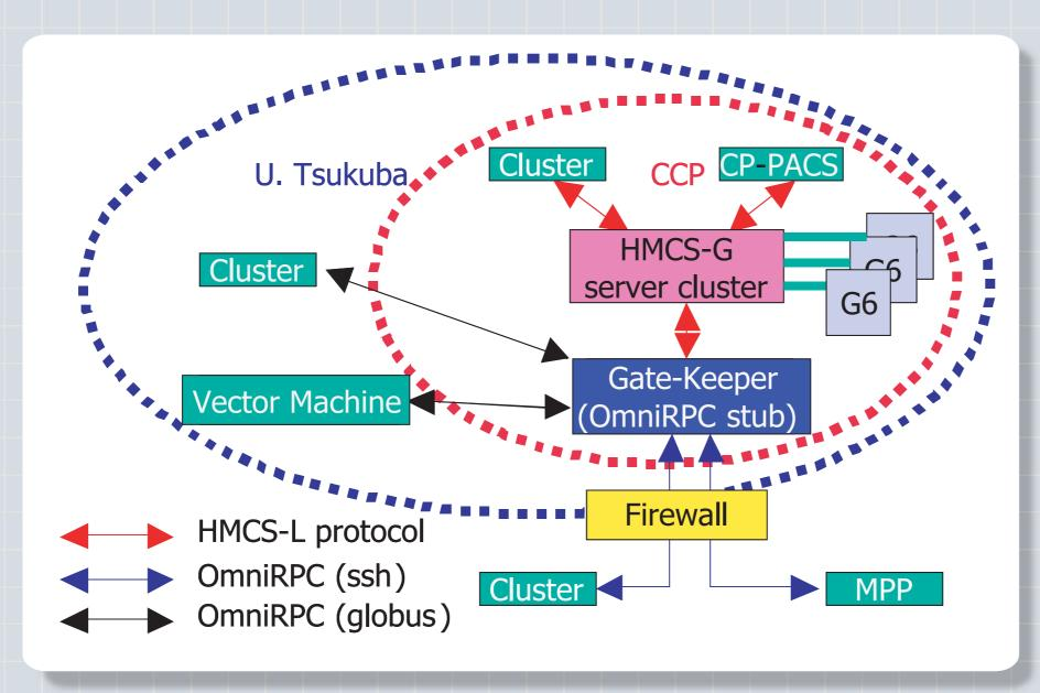
HMCS-G is a gravity calculation service system centering HMCS server with GRAPE-6 gravity engine with GridRPC which enables world-wide access to
