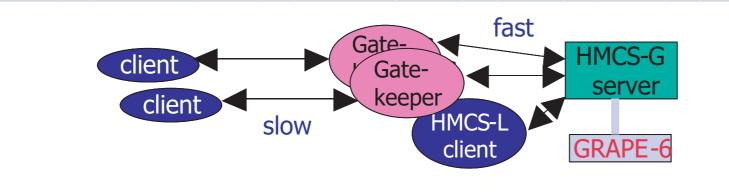
OmniRPC Agent works as communication buffer to absorb the speed-gap between WAN and LAN.
