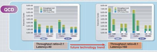
SCIMA is robust to large throughput ratio and long memory access latency caused by current technology trend of CPU-memory speed gap
