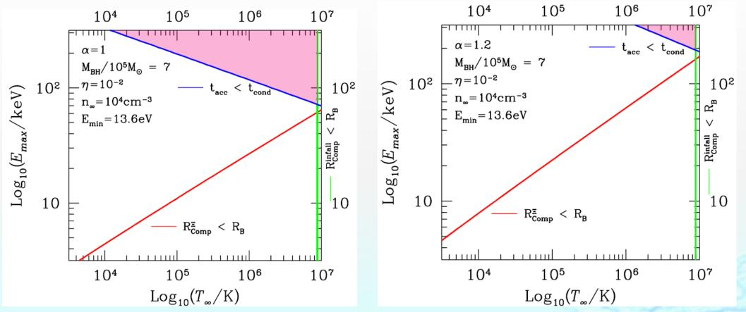
high  $E_{\text{max}}$ , flatter spectrum of irradiation  $\rightarrow$  high  $T_{\text{C}}$  $\rightarrow$  efficient conductive heating
